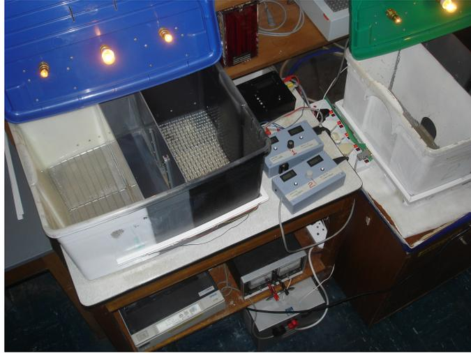
Figure 2.1: CPP Boxes with open lids, counters in between, the transformer for the DC lights and the printer below
